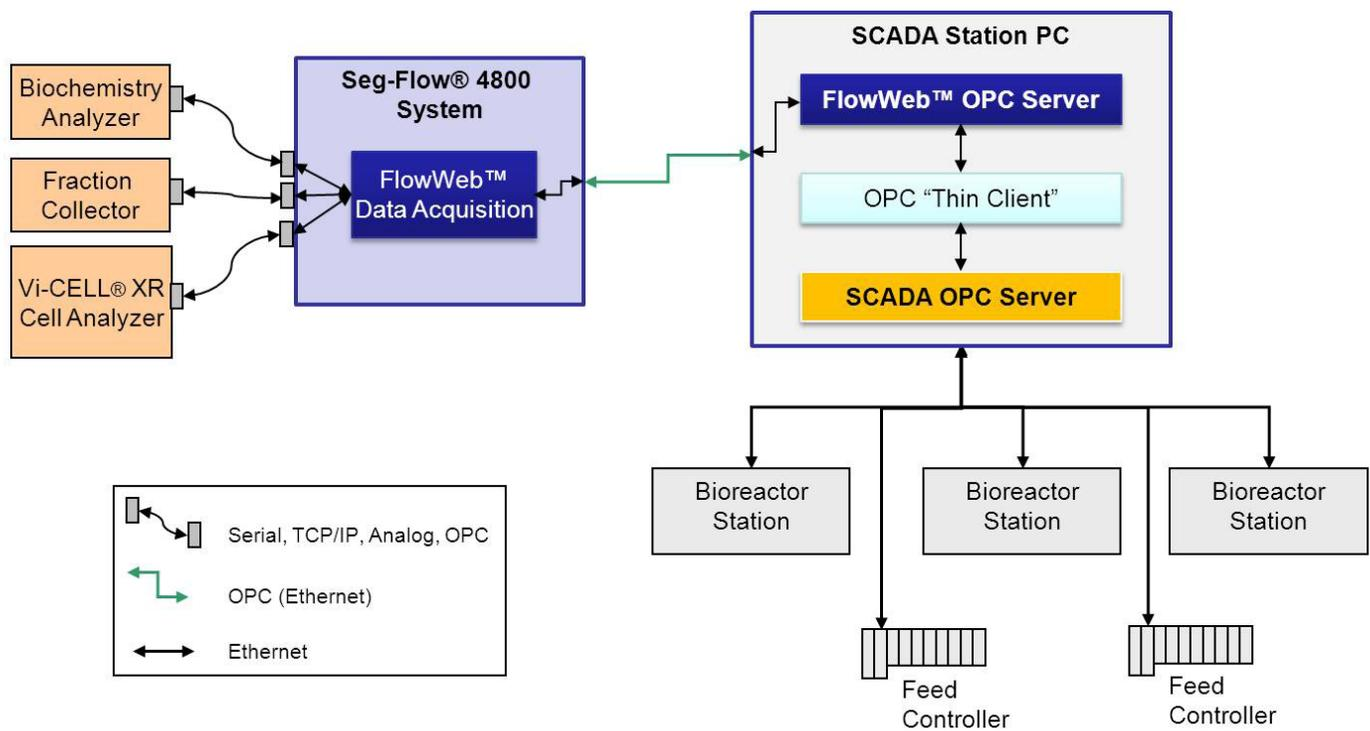
**Figure 2.** Architecture for the Vi-CELL XR/Seg-Flow integrated bioprocess PAT solution. The Vi-CELL XR/Seg-Flow interface can be integrated with additional third-party analytical technologies to provide a complete PAT solution for cell culture monitoring and control.
